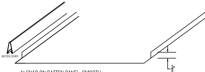
1" SNAP ON BATTEN PANEL, SMOOTH 12", 16", 18", AND 20" WIDE PANEL PRE-NOTCHED
