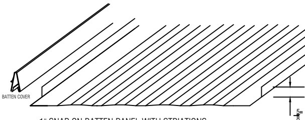
1" SNAP ON BATTEN PANEL WITH STRIATIONS 12", 16", 18", AND 20" WIDE PANEL PRE-NOTCHED
