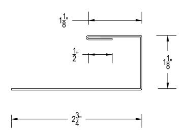
FLUSH SEAM SOFFIT J-CHANNEL
